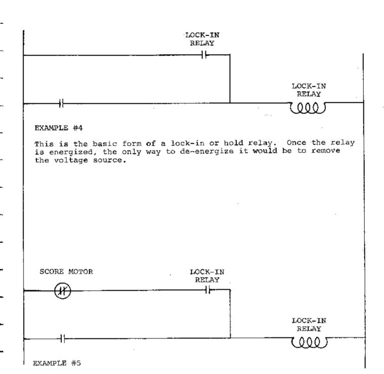
This lock in circuit will drop out when ever the score motor turns. The score motor switch is usually a #8 or #10 cam switch.
