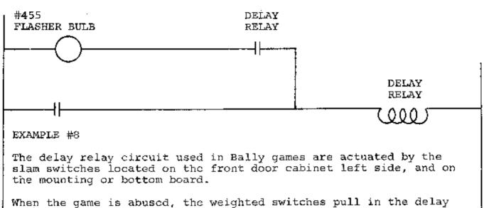
When the game is abused, the weighted switches pull in the delay relay. The relay is locked in by the filament of the flasher lamp. As the filament of the lamp heats up, the internal bimetal contacts open the lamp circuit causing the relay to drop out.
