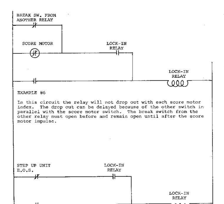
The relay is locked in through a step up unit end of stroke switch. The step up unit must advance for the relay to drop out. A typical example of this circuit is in the point relay (10,100,1000) lock in circuits.
