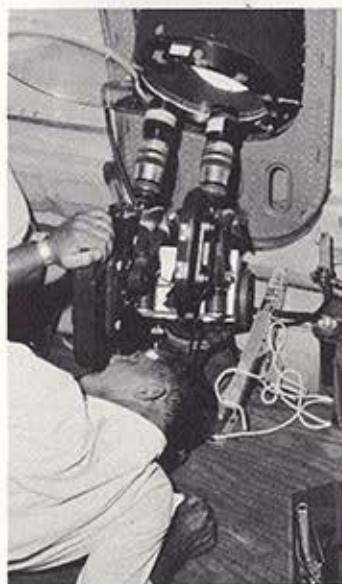
One Arriflex 35 and one Arriflex 35S, both fitted with Kinfitt telephoto lens and dual mounted amidships, positioned to shoot the sun.
